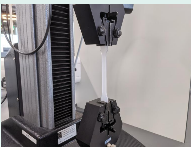
Tensile testing on a tensometer
