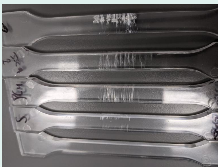
Crazing and cracking after exposure
