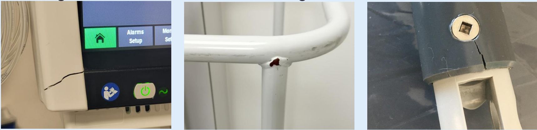
Damage observed on in-service healthcare equipment: cracking of plastic housings, frames and fittings following routine cleaning and disinfection.
