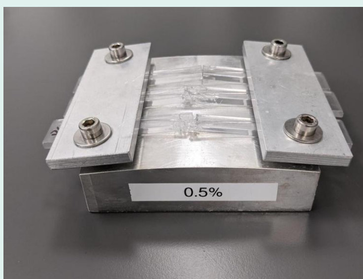
Specimens held at 0.5 % strain
